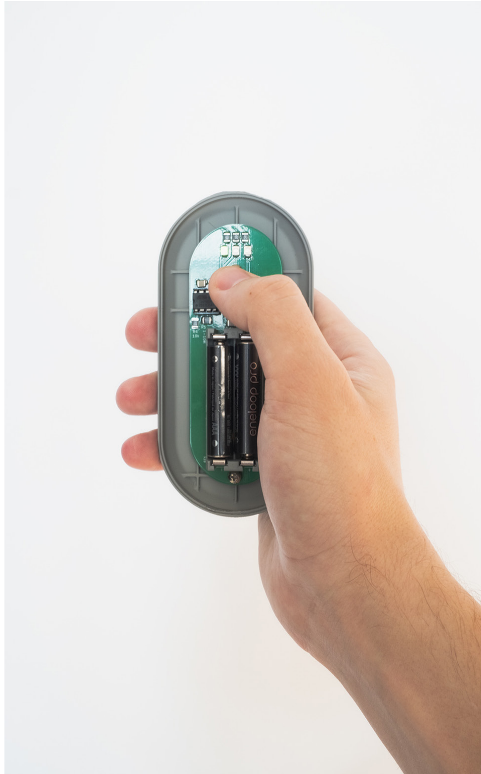
PCB prototype validated the single LED/button interaction, component layout and fit within the FDM prototype.
