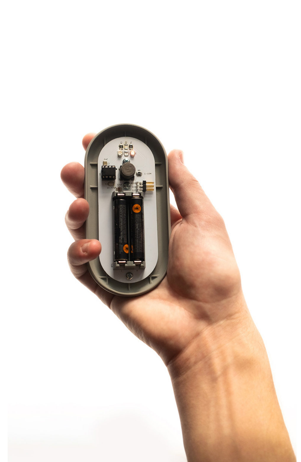
PCB revision refined component layout and BOM, swapped button for improved tactile click, and increased board size to improve space between edge and screw hole.
