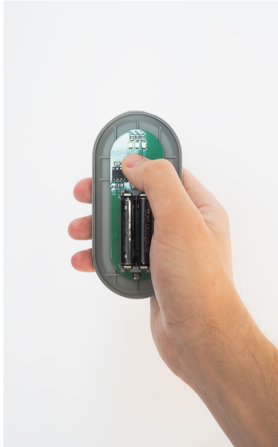
PCB prototype validated the single LED/button interaction, component layout and fit within the FDM prototype.
